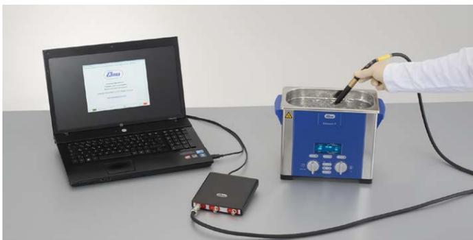
*Elmasonic P 30 H during the cavimeter test*
