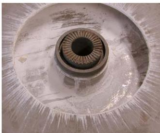
*Contaminated and corroded powdering equipment*
