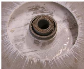
*Contaminated and corroded powdering equipment*
