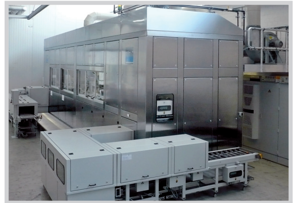
Fully encapsulated cleaning facility in clean room
