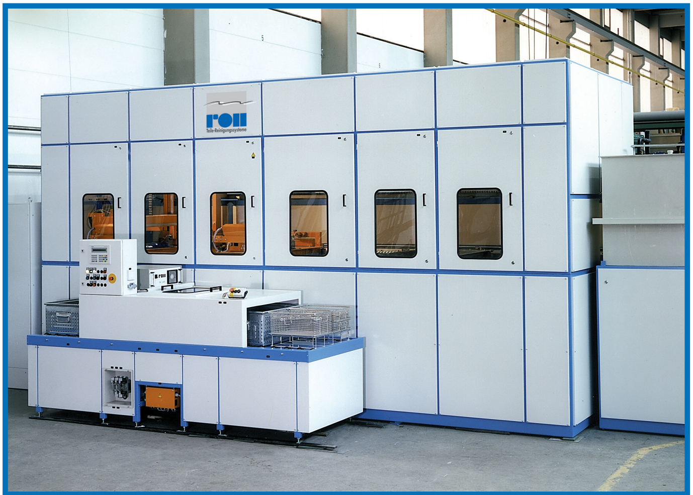
Multichamber immersion facility with several basket holders
